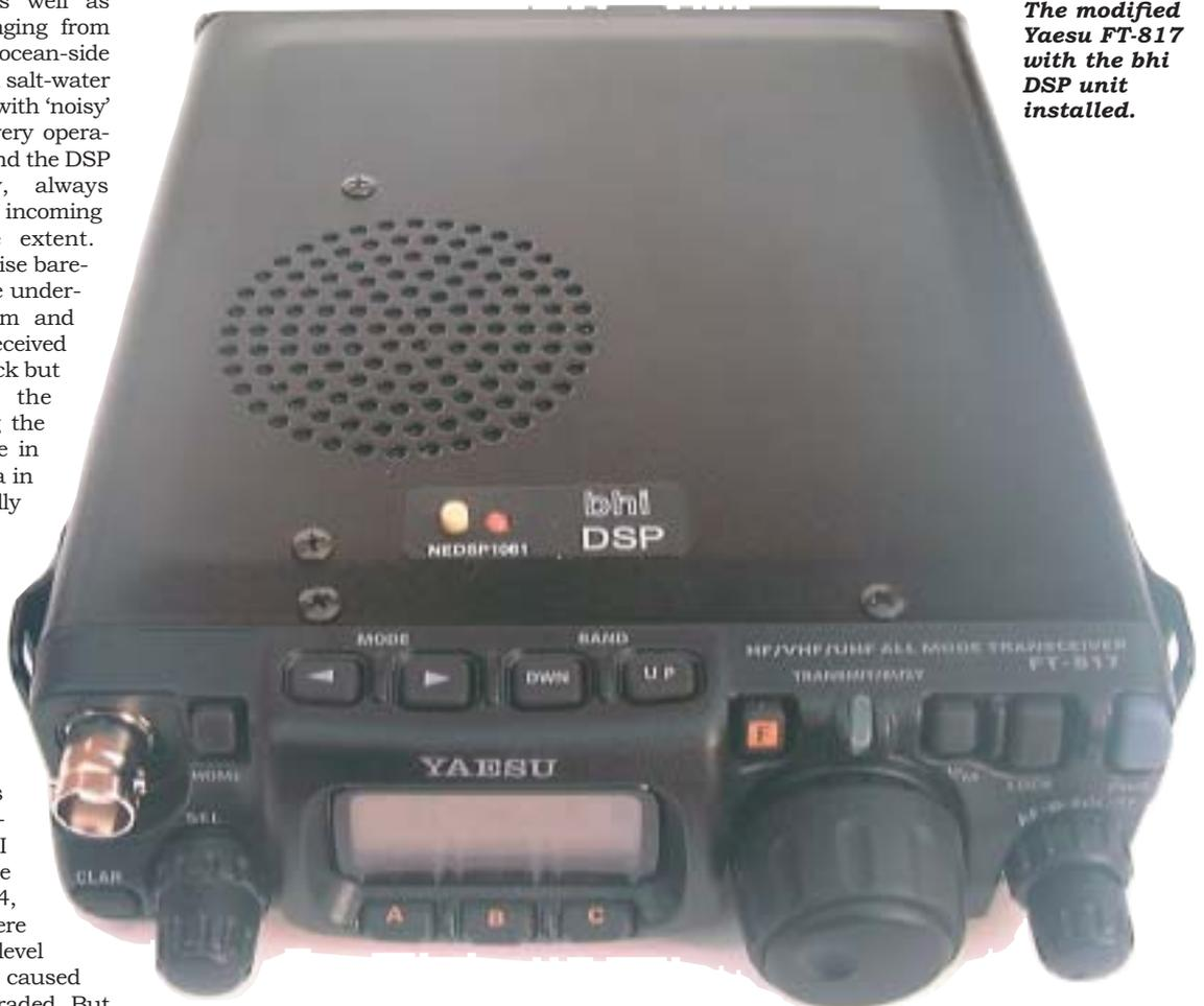
**The modified Yaesu FT-817 with the bhi DSP unit installed.**
