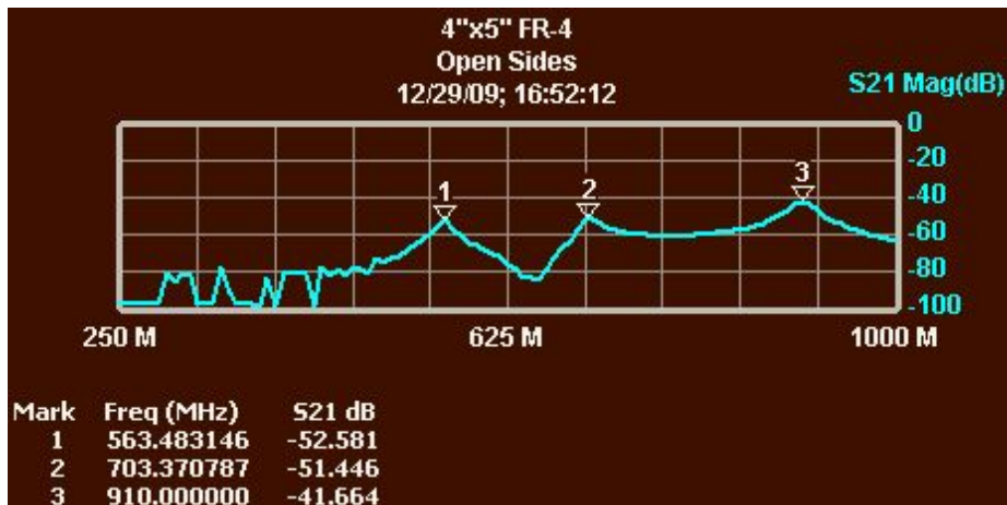
Figure 2—Transmission of FR-4 from corner to corner
