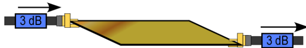
Figure 1—PCB Transmission Test Setup For FR-4, the connectors were vertically mounted without legs, with the center pin projecting through the board but not attached to the other side.
