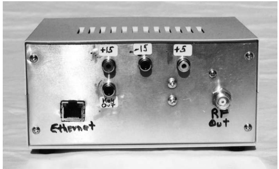
Figure 4 — This photo shows the back panel of the exciter, with the various input/output connectors.
