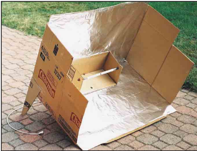
Figure 11 —The completed high-performance corner reflector. Note how the box corners hold the reflectors and dipole feed in place. The rear legs set the antenna elevation to 20°—this gives good coverage at the author's latitude.
