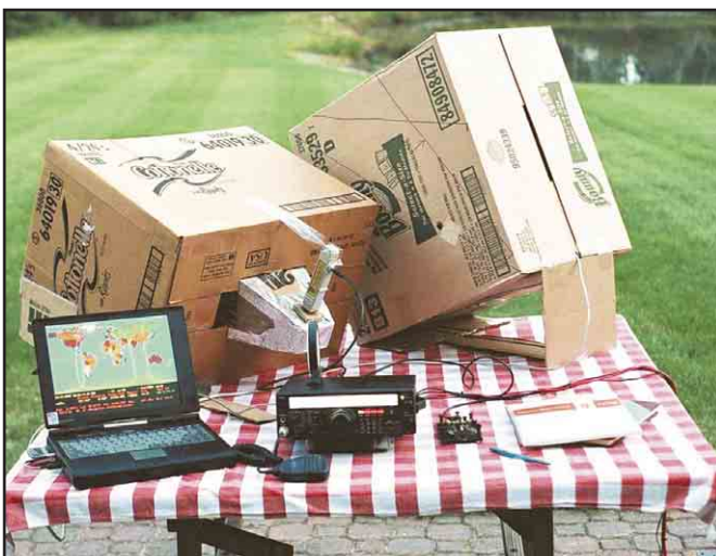
Figure 13 —The complete satellite station with the tracking laptop, FT-847 transceiver, and both downlink and uplink antennas. [Recognize that key? It's a J-38 from 1944, bridging a gap of almost 60 years!—Ed.]
