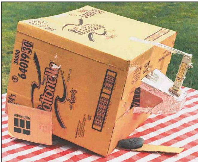
Figure 5— Side view of the downlink pyramidal horn showing the elevation control supports and how the downconverter is attached to the horn. The downconverter is pulled forward by the tape to align the probe wire parallel to the rear surface of the horn.
