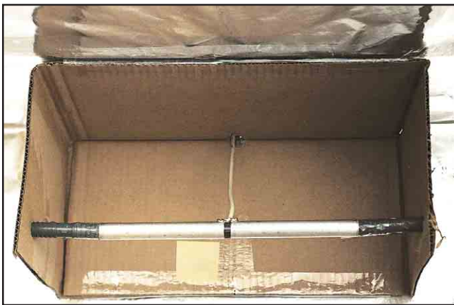
Figure 12 —A close-up of the high-performance corner reflector dipole feed.
