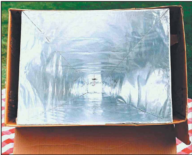
Figure 4— Front view of the downlink pyramidal horn showing how it is mounted in the support carton. Notice the coax probe at the back of the horn.
