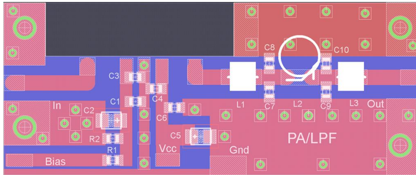
Fig2 Component overlay for the 144MHz amplifier module with LPF. C8 and C10 are not used in this version of the amplifier module.
